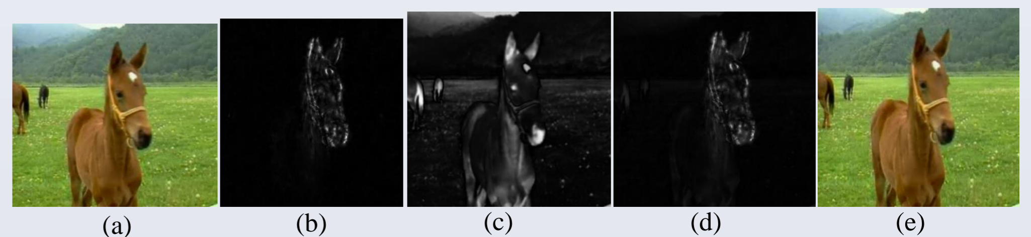
Fig. 3. a) Original Frame (medium content), b) Motion Map, c) Frequency Tuned Map, d) Saliency Map, e) Encoded Frame containing secure data
