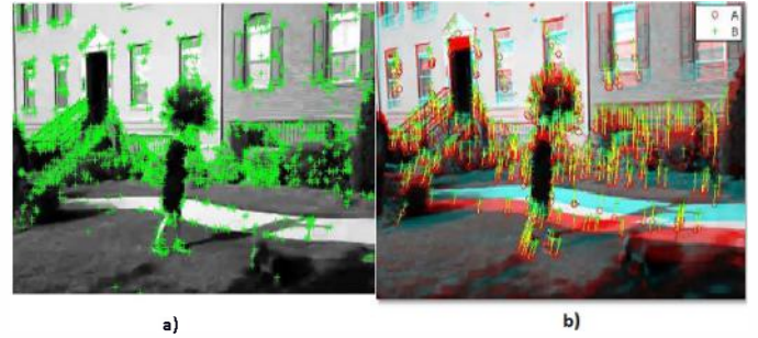
Fig. 3. (a) Corners detected by FAST algorithm (b) Corresponding features between frame A and frame B. Features of frame A are marked green and features of frame B are marked red
