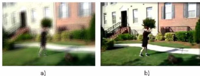
Fig. 6. (a) Mean of 10 original input frames (b) Mean of 10 corrected frames
