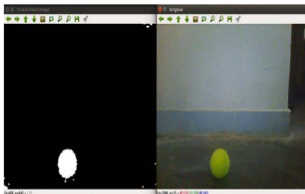
Fig. 5. Figure shows the original and the thresholded images of an object with no occlusion and under indoor environmental conditions.
