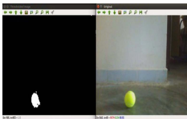
Fig. 6. Figure shows the thresholded image of the same object with no occlusion but with a variation in the ambient light. Due to this the thresholded image does not truly represent the original object. But the algorithm successfully achieves to recognize the object by assuming the position of the current object to be in the vicinity of the original object in the subsequent frames of a video and therefore not losing track of the object due to ambient light effects.
