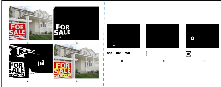
Fig. 2. Left Column: (a) Original image (b) Bright regions (c) Dark regions (d) After processing on these regions final set of blobs detected by eMSERs; Right Column: Top Row: (a)-(c) eMSER region; Bottom Row: (a) Binarized region obtained from original image (b) Binarized region neglected due to size constraints (c) binarized image-refined object (alphabet) obtained with less disturbance which gives us better results
